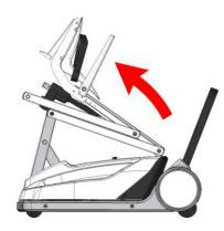
Align the mounting holes (A) of arms, frame and actuator.
