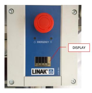
To check the status of charge of the battery is enough to check the lighting of the light switches placed on the display.
